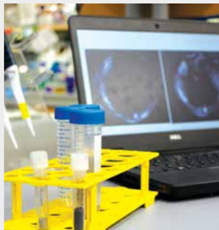
The novel contrast agent (grey solution in larger tube) was developed using nanodiamonds and provides clearer MRI images of liver tumours at lower dosages
