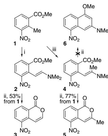
**Scheme 1.** Condensation of methyl 2-methyl-3-nitrobenzoate **1** with DMF–DMA (Ref. 4) and with DMA–DMA (Ref. 5), followed by different modes of cyclisation. Reagents: (i) HC(OMe)<sub>2</sub>NMe<sub>2</sub>, DMF,  $\Delta$ ; (ii) SiO<sub>2</sub>, EtOAc and (iii) MeC(OMe)<sub>2</sub>NMe<sub>2</sub>, AcNMe<sub>2</sub>,  $\Delta$ .
